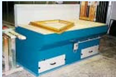
Sanding table for de-nib sanding.
