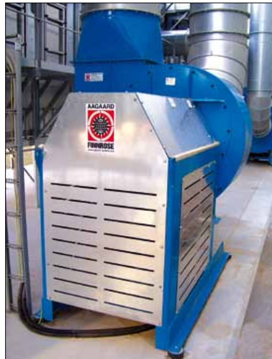
Agaard manufactures direct-driven and indirect-driven medium-pressure material transport fans.
